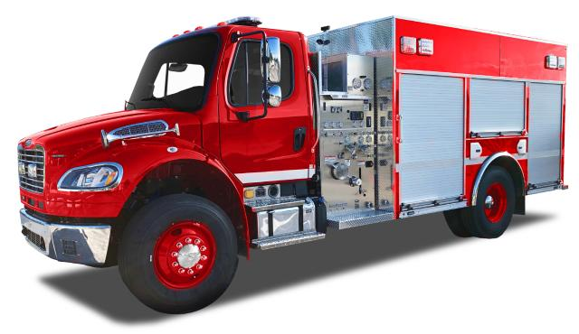
All-aluminum, huck-bolted body designed for long-term durability and maximum storage capacity. This technology provides a lightweight body without sacrificing structural integrity. The design has been verified with stringent Finite Element Analysis (FEA) where the body is stressed to the maximum chassis Gross Vehicle Weight Rating (GVWR) and off-road frame twisting to assure long-term durability.
